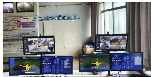
条形煤场斗轮堆取料机无人值守
